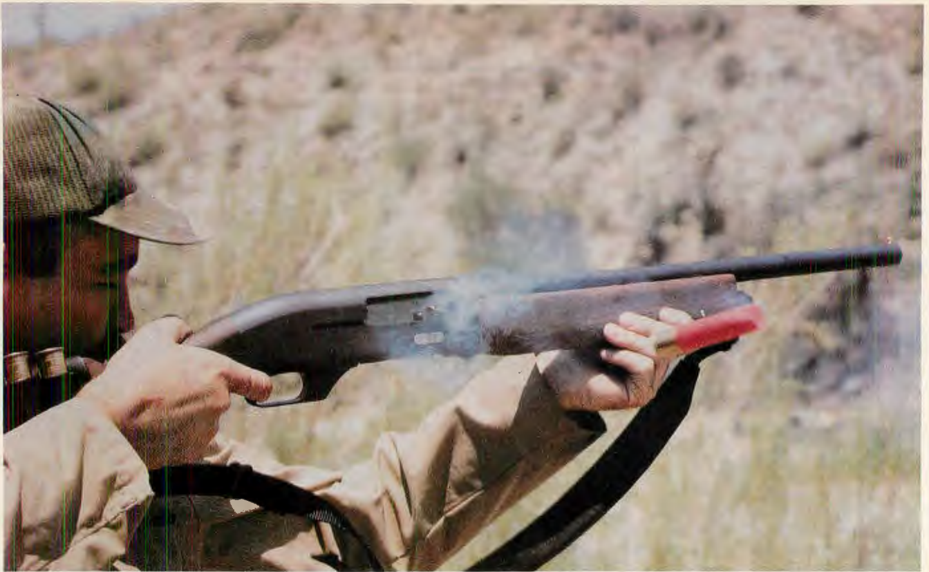
ABOVE: MAG-10's muzzle-heavy design helps it follow targets, and thick recoil pad and high weight keep recoil manageable.
